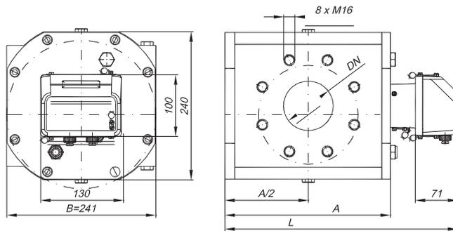
fig.5 Dimensions of the CGR Rotary Gas Meters
