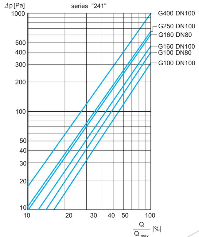
fig. 6 Diagram of pressure loss related to  $\rho = 1,2 \text{ kg/m}^3$
