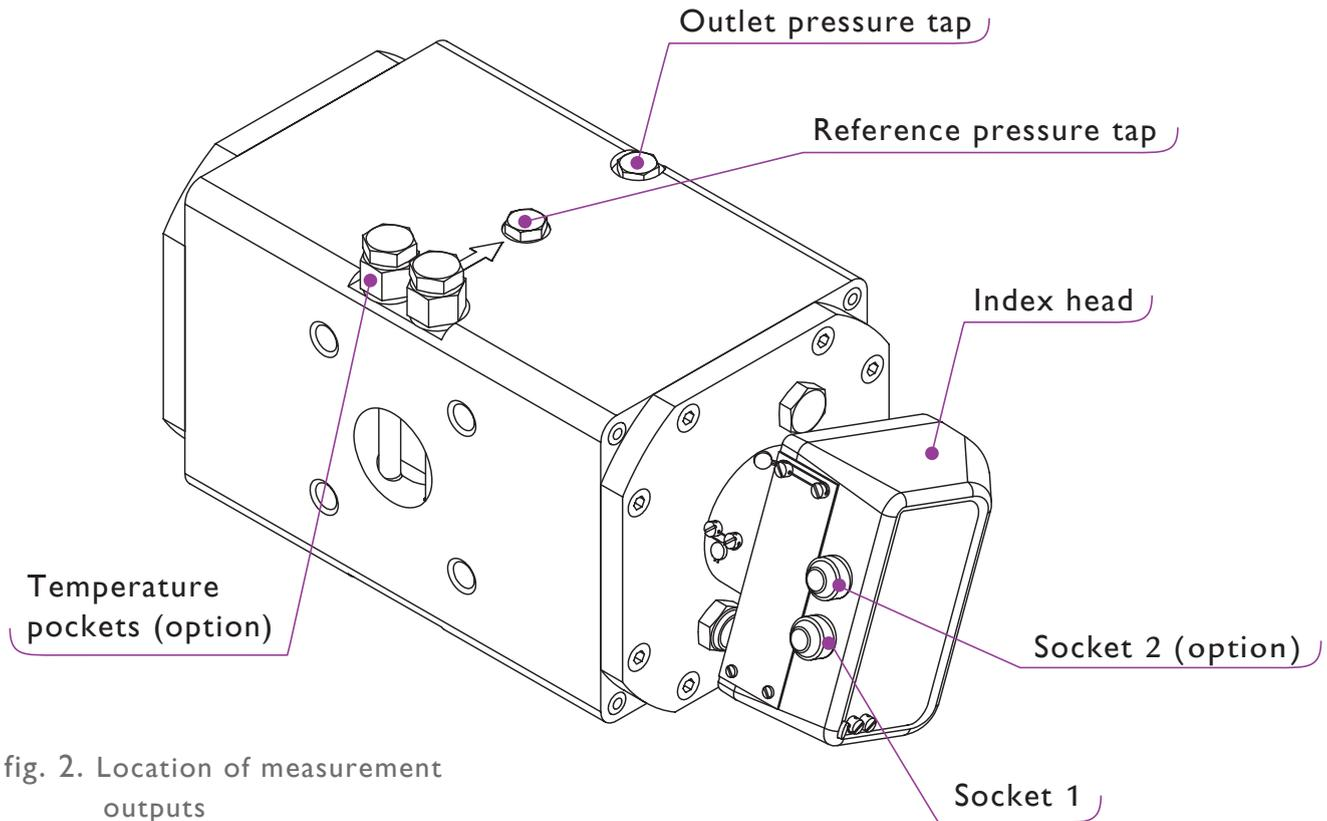
fig. 2. Location of measurement outputs
