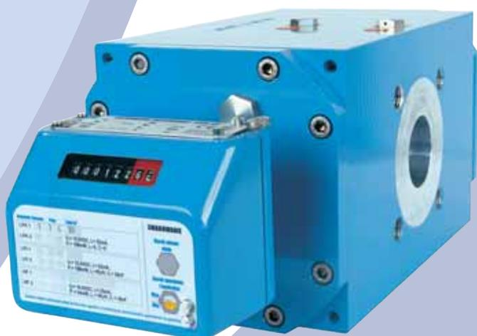
The rotary gas meters are positive displacement meters, designed to measure quantity of gas, for custody transfer or technical measurement applications. The devices are mainly applied for gas flow ranges from 0.2 up to 650 m<sup>3</sup>/h, and the pressure range up to 20 bar. Special design rotary gas meters may also be used in higher pressure installations.
